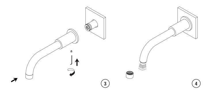
Install spout to the ffixing pipe and attach it with set screw.
