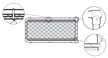
Fasten the post hinges "N" (hinge with the pin) to the vertical post that you are hanging the gate on approx. 8-12 inches from top & bottom. The top post hinge should point up, and the bottom post hinge should point down.
