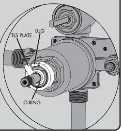
16 Reinstall Rough-In Template over Valve to protect it during final wall preparation.
