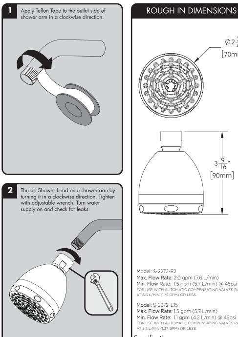
3<u>7</u>16 [90mm] Max. Flow Rate: 2.0 gpm (7.6 L/min) Min. Flow Rate: 1.5 gpm (5.7 L/min) @ 45psi FOR USE WITH AUTOMATIC COMPENSATING VALVES RATED AT 6.6 L/MIN (1.75 GPM) OR LESS.
