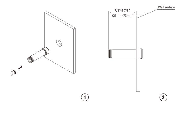
Install the fixing pipe to elbow located in the wall cavity.
