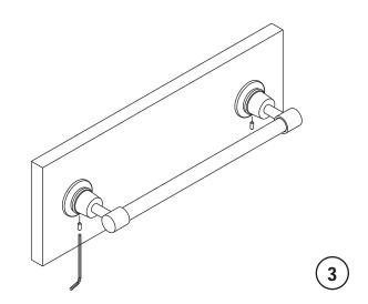
**3** Place assembly over the mounting bracket with set screws facing down. Tighten the set screws.
