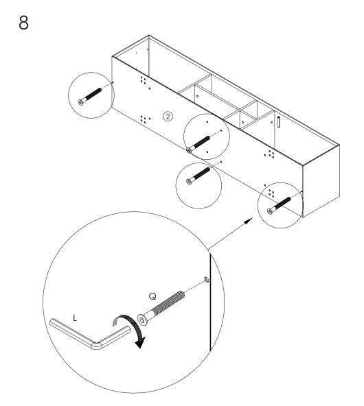
During assembly, hand tighten screws only. When the screws are in place, tighten completely.
