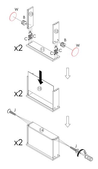
During assembly, hand tighten screws only. When the screws are in place, tighten completely.
