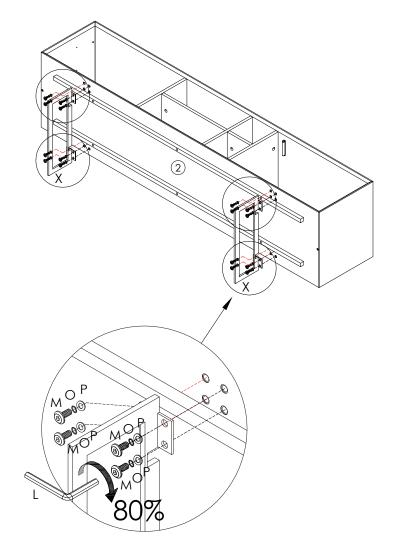
During assembly, hand tighten screws only. When the screws are in place, tighten completely.
