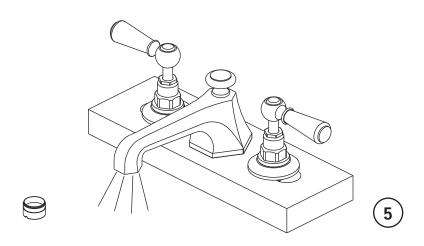
After installing faucet, open the hot and cold supplies to check for leaks. Turn on faucet handle for one minute to flush debris from faucet. Turn off the handle.
