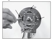
Remove four mounting screws from Motor Housing where indicated to use for Rear Grille in Step 7.
