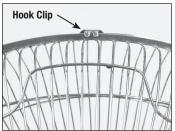
Attach Front Grille to Rear Grille with Hook Clip centered on the top above Wire Handle.
