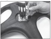
Assemble Extension Pole onto Base by inserting 4 ea. 2-1/2" bolts through openings.
