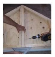
Fasten panels H&I to each other. Make sure they are even on the bottom. Fasten. Piece may bow slightly, this can be made straight in the following steps.
