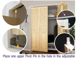
bracket (L) and the other upper Pivot Pin into the groove on the Track (B). Lift the door assembly and drop the lower pin into lower bracket slot (D).
