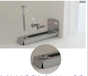
Mount bottom bracket (Part D) to the wall jamb using two screws (Part C) so the center of serrated hole is aligned vertically with the center of the Top Track. Be sure bracket is seated firmly to the floor then fix it using one screw (Part I). Use this screw for wood flooring only. Press down into carpet if necessary.
