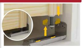
To adjust for height, lift door from Bottom Bracket (Part D) and rotate Knur-led Hinge Pin (Part F) clockwise to raise the door and counter-clockwise to lower it. Verify there is at leat one quarter inch of clearance between the pivot door and the jamb.
