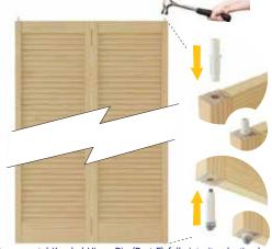
Screw metal Knurled Hinge Pin (Part F) fully into its plastic sleeve first, to prevent damaging sleeve when tapping with hammer. Then, insert the entire set into the lower socket of door panel, tapping lightly with hammer to fully seat. Once seated, back-out pin approximately 1/4". Now insert the two Plastic Top Pivots (Part G) and tap-in lightly to fully seat.
