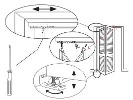
Square-up doors in the opening and tighten set screw on sliding-hinge bracket in the Top Track (Part B) to fix door position. Test-close doors to be sure they operate smoothly. Doors should have equal space on all sides. Verify there is at leat one quarter inch of clearance between the pivot door and the jamb.
