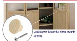
Install the Pull Handle (Part H), by drilling a 3/16" (5mm) hole in the center of the Guide Door. Insert a long screw (Part I) from back and fasten knob.
