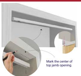
Mark center of top jamb at each side of opening and center point. You will use these marks to align Top Track.
