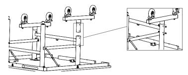
5. With two people, flip the assembly over, being careful not to bend the Supporting Braces, then remove the blanket or cardboard. Repeat this step on the other half of the assembly.
