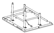
3. Pull up on the braces to lock the legs into position.
