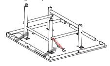
4. Slide (2) Wheel Assemblies into the slots in the legs, then attach them using (8) Bolts. Repeat this step on the other half of the assembly.
