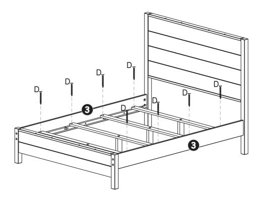
**Note:** there are no pre-drilled holes for screws D on part 3.
