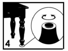
Some furniture comes with height adjustement knobs underneath each leg. To lower or to raise each leg, you need to turn clockwise or counterclockwise, respectively.
