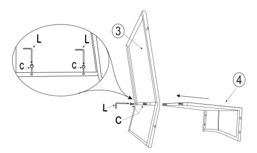
Step 1: Insert seat panel (4) into the two holes on chair back (3), then secure them with 2 screws (C) by using allen wrench (L). Do not tighten all screws now.
