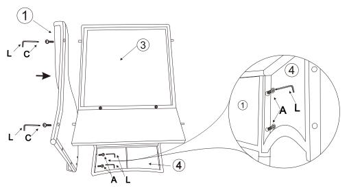
Step 2: Secure left arm (1) to assembled chair back (3) with 2 screws (C) by using allen wrench(L). Do not tighten all screws now. Then, secure seat panel (4) to assembled left arm (1) with 2 screws (A) by using allen wrench (L). Do not fully tighten now.
