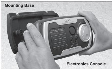
A. Separate Mounting Base From Electronics Console.
