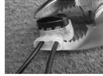
2. Using pliers squeeze the top black button down solidly until it bottoms out.
