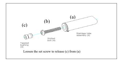
Parts included with unit: Allen wrench (1) Philips screws #8 x 2.5" (4) Tapered Bushing - c (4) Slotted Bolts - b (4) Stainless Tube Assembly - a (4) Marking Disc (1) Cover plate (1) Screws for Cover plate (2) Wire Connectors suitable for 12-16 AWG wire (6)
