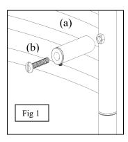
Remember: Unit should not be mounted closer than 2 inches below an overhanging surface (i.e. shelf) and no closer than 1-1/4 inches above the floor and/or baseboard.
