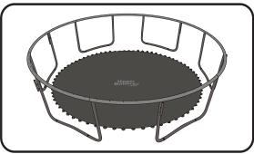
**Step 2**Hook the galvanized hooks onto the trampoline mat edges, as shown in figure.
