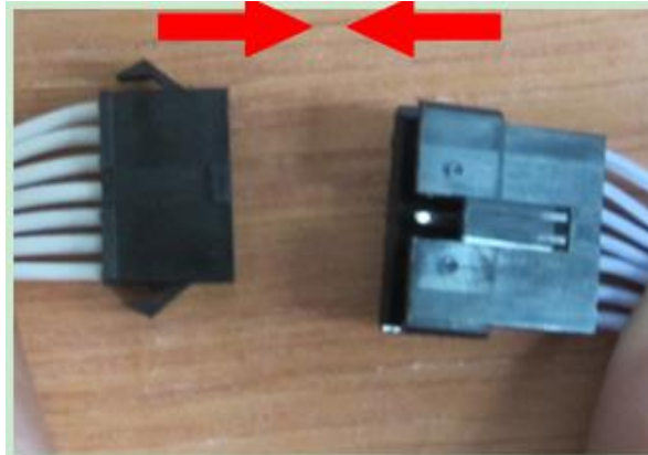
FIG 16 Connecting control panel connectors
