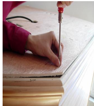
FIG 18.1 Screw down Roof Cover
