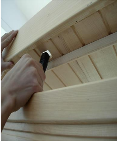
FIG 12 Slip cords/wires through corresponding holes
