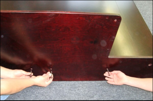
Attach tray ends (be sure to note there is a left and right side.)
