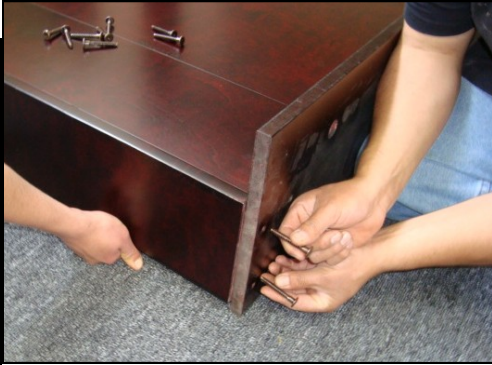
Attach tray ends (be sure to note there is a left and right side.)
