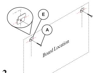
Attach Z-Hangers (E) using Long Screws (A) as shown.
