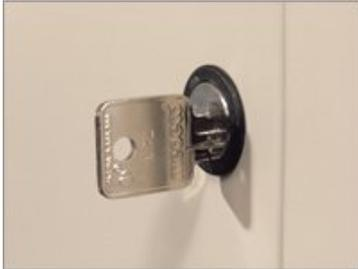
**Key Lock-** This 4-pin key lock comes standard on most FireKing Files. A single lock can secure up to 4 drawers, or individual locks can be installed on each drawer in a file. Drawers can also be controlled by setting the drawer catches, which lets the user decide which drawers are to be locked.
