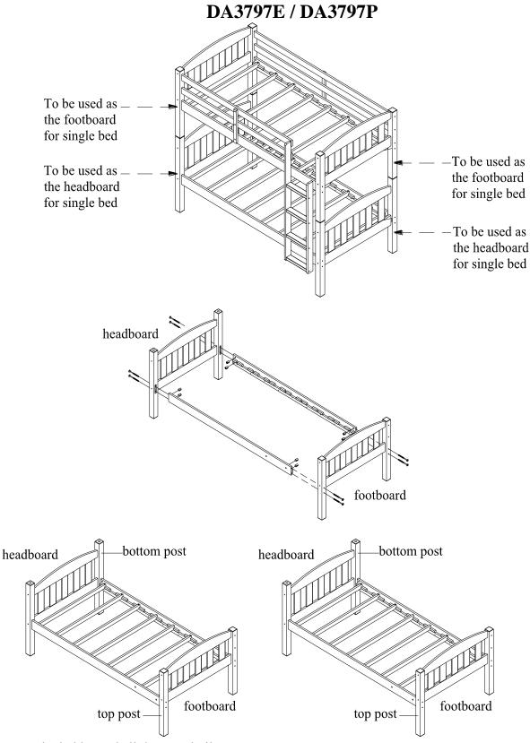
Remove the ladder and all the guardrails.
