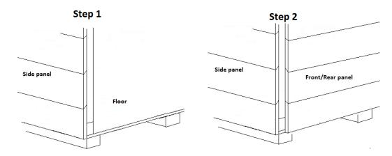
**Step 1**. Position the first side panel so that the edge of the panel is flush with the edge of the floor and the overhang on the bottom of the panel is butted up to the floor.
