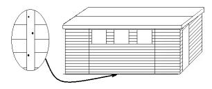
Place the joining strips over the front, rear and sides joins in the panels and fix into place with 30mm nails.
