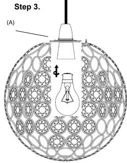
**Step 3.** Re-fit the shade fixing ring to secure the pendant on the lamp holder, do not over-tighten. Install the bulb.
