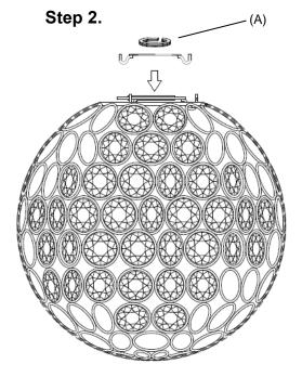
Step 2. If your current pendant lamp holder is a standard Bayonet cap lamp holder type (B22/BC) the shade reducer (A) will need to be positioned on the pendant frame (gimble) to reduce the shade hole size.
