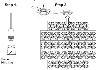
**Step 1.** Remove the shade fixing ring from the lamp holder.
