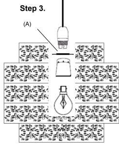
**Step 3.** Re-fit the shade fixing ring to secure the pendant on the lamp holder, do not overtighten.
