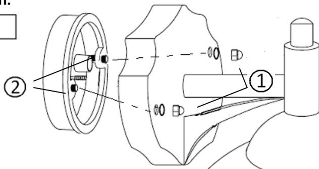
1. Determine the position of your light fitting taking into account the exit position of the cable. Ensure that the mounting surface is solid, preferably a brick or block wall and ensure that there are no other cables or pipes beneath the surface. Use appropriate fixings. Wall plugs and screws as supplied are shown here.
