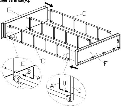
2 Assembly the Shelf(G) onto the Side Frame(C) and using the Bolt(B) by Allen Wrench(A).
