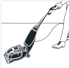
When machine is reclined brushbar will power. Upright position brushbar will not power.
