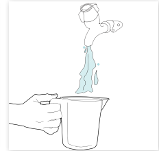
Mix the solution with warm water (max 40° C) and fill tank with solution.
