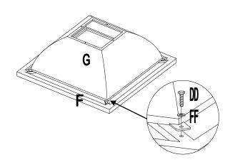
2. Put Bowl Base (G) on reverse side of Table Top (F), then use Bolt (DD) and Flat Washer (FF) to lock tightly by wrench (GG). See as Fig. 2.
