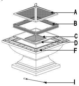
4. Turn over the assembled fire pit to make Table Top (F) on the top, then put Bowl (D), Grate (C) and Square Screen (A) in turn. Put Poker (I) on the side. **Now, fire pit is ready to use!**
