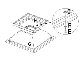
3. Put Base (H) on the Bowl Base (G), then use Bolt (EE), Flat Washer (FF) and Nut (CC) to locking tightly by Wrench (GG). See as Fig. 3.
