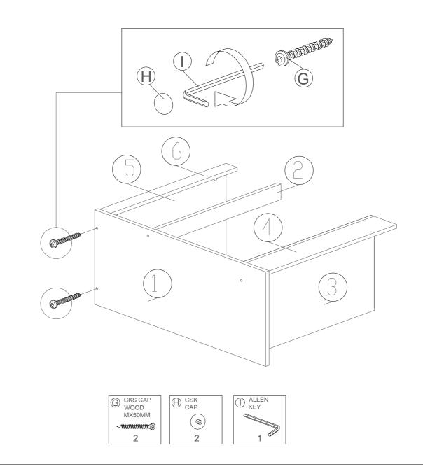
Fix Panel (6) onto panel(5) by inserting minifix (M1) into panel (5)'s L-thru holes and using allen key (I) to tighten it after that insert minifix cap(H).
