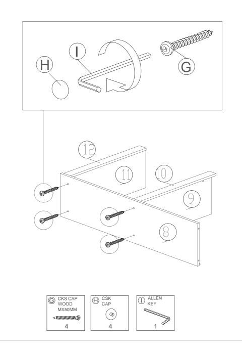
Fix Panel (9,11) onto panel(10,12) by inserting minifix (M1) into panel (9,11)'s L-thru holes and using allen key (I) to tighten it after that insert minifix cap(H).
