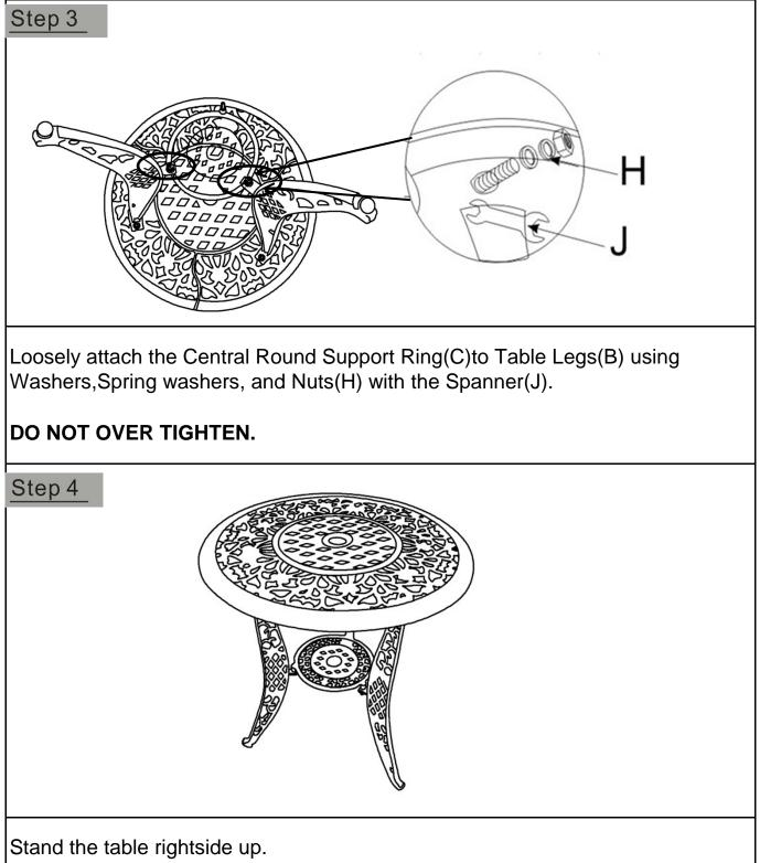
Adjust the Legs pre-installed Levellers until the table is level with the ground. After the table is completely level, in a sequential manner, tighten up all the bolts.
