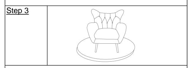
Place the chair on a LEVEL SURFACE to see if it wobbles. If it wobbles, press firmly down on both armrests at the same time. This will help to ensure all Bolts and gaps reach full alignment status.
