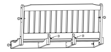
3) Attach the braces to the back with two B bolts
