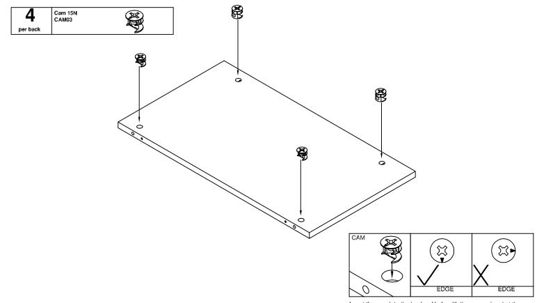
Insert the cam into the 'surface' hole with the arrow aimed at the adjacent edge which has the smaller hole.
