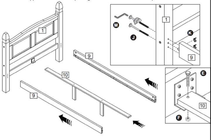
Step 7: Join the two sections together using hardware parts J, K and M. Secure the centre rail (10) using hardware parts E and F.
