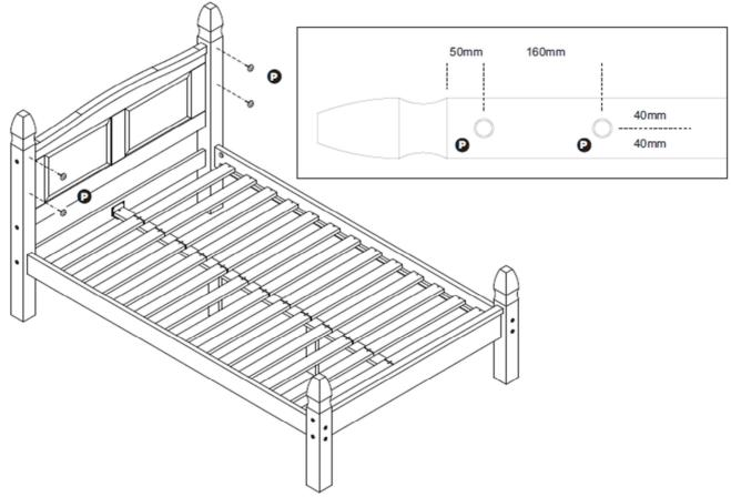
Note: When everything has been assembled, tighten all bolts and attach the wooden buttons to the holes on the bed posts
