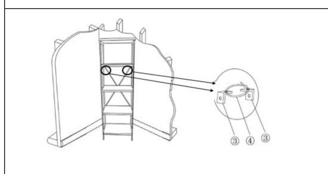
**C:** Move the Console against the wall. Then pull the Bookcase Restraint Strap(④) through two Metal Brackets(③) one by one, lock tight the Bookcase Restraint Strap(④), as shown above. Bookcase Restraint Device is installed and Console is ready for use.
