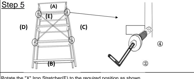
Rotate the "X" Iron Stretcher(E) to the required position as shown. Attach "X" Iron Stretcher(E) to the Bookcase(E) using Bolt(④) with Allen Key(②). **Only loosely tighten the Bolts.**
