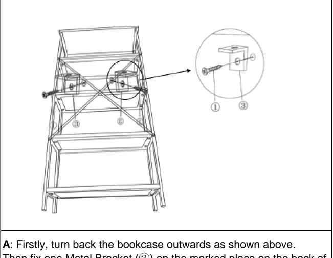
Then fix one Metal Bracket (③) on the marked place on the back of console by the 2.0cm Self Tapping Screw(①). The mark will be different based on products.
