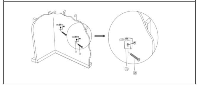
**B:** Find out the screw holes on the wall. First, mark the point at same height as L-shaped Metal Bracket (③) on product. You can find these same points in two ways as below:
