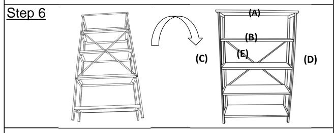
Tighten all Bolts, And Stand the Console up as shown. Then Check for stability .
