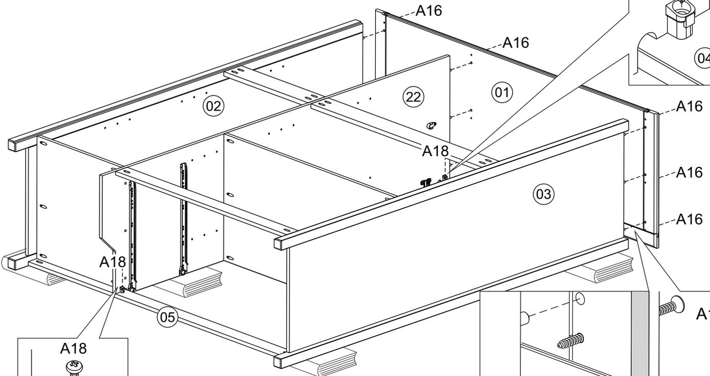
Attention: There are no predrilled holes for the A16 screws on parts 02, 03 and 22.
