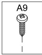
Attention: There are no predrilled holes for the A9 screws on parts 06, 07 and 25.
