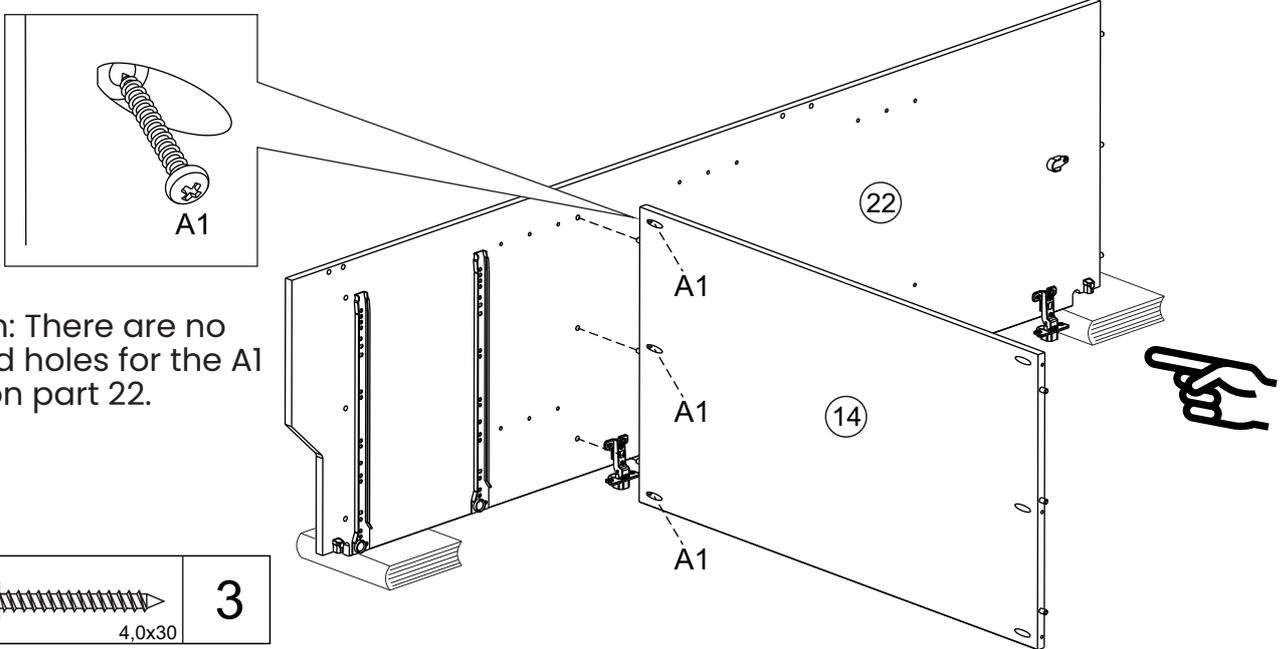
Attention: There are no predrilled holes for the A1 screws on part 22.
