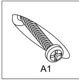
Attention: There are no predrilled holes for the A1 screws on part 22.
