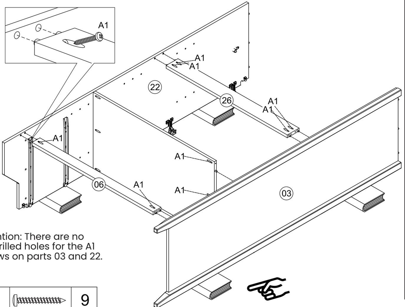
Attention: There are no predrilled holes for the A1 screws on parts 03 and 22.
