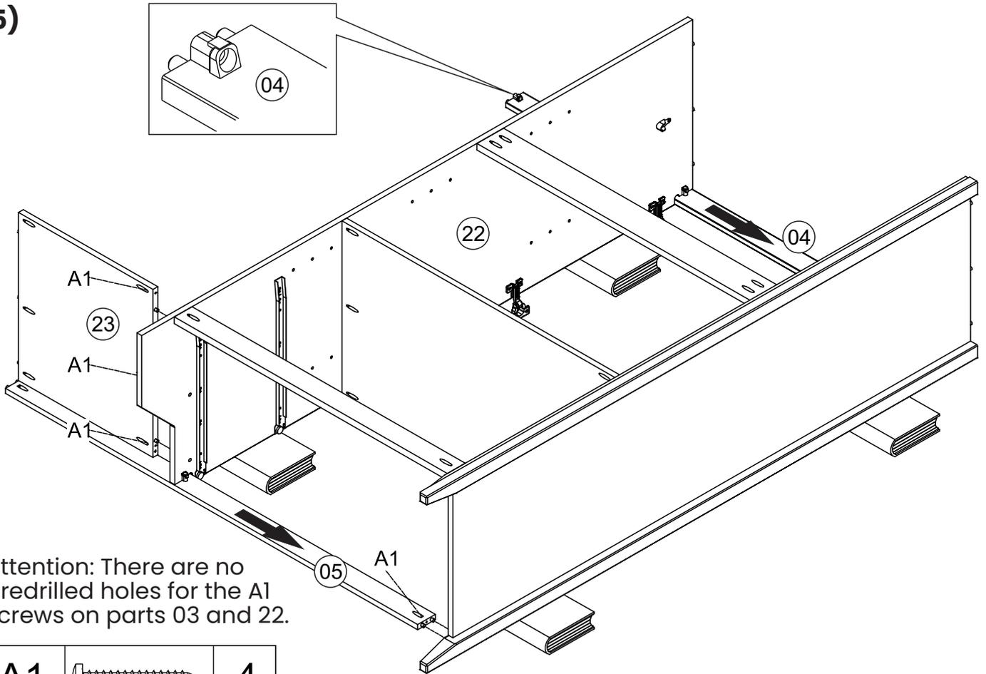
Attention: There are no predrilled holes for the A1 screws on parts 03 and 22.
