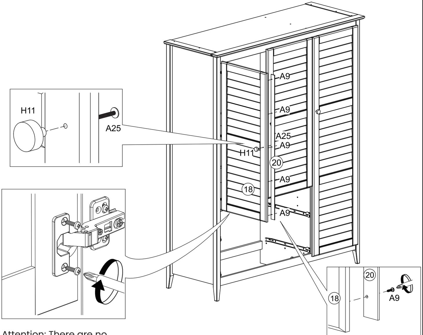
Attention: There are no predrilled holes for the A9 screws on part 18.
