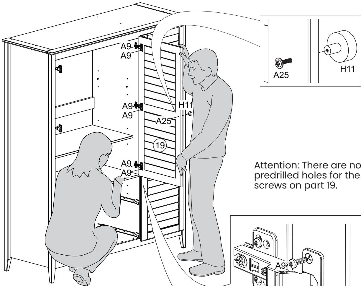
Attention: There are no predrilled holes for the A9 screws on part 19.
