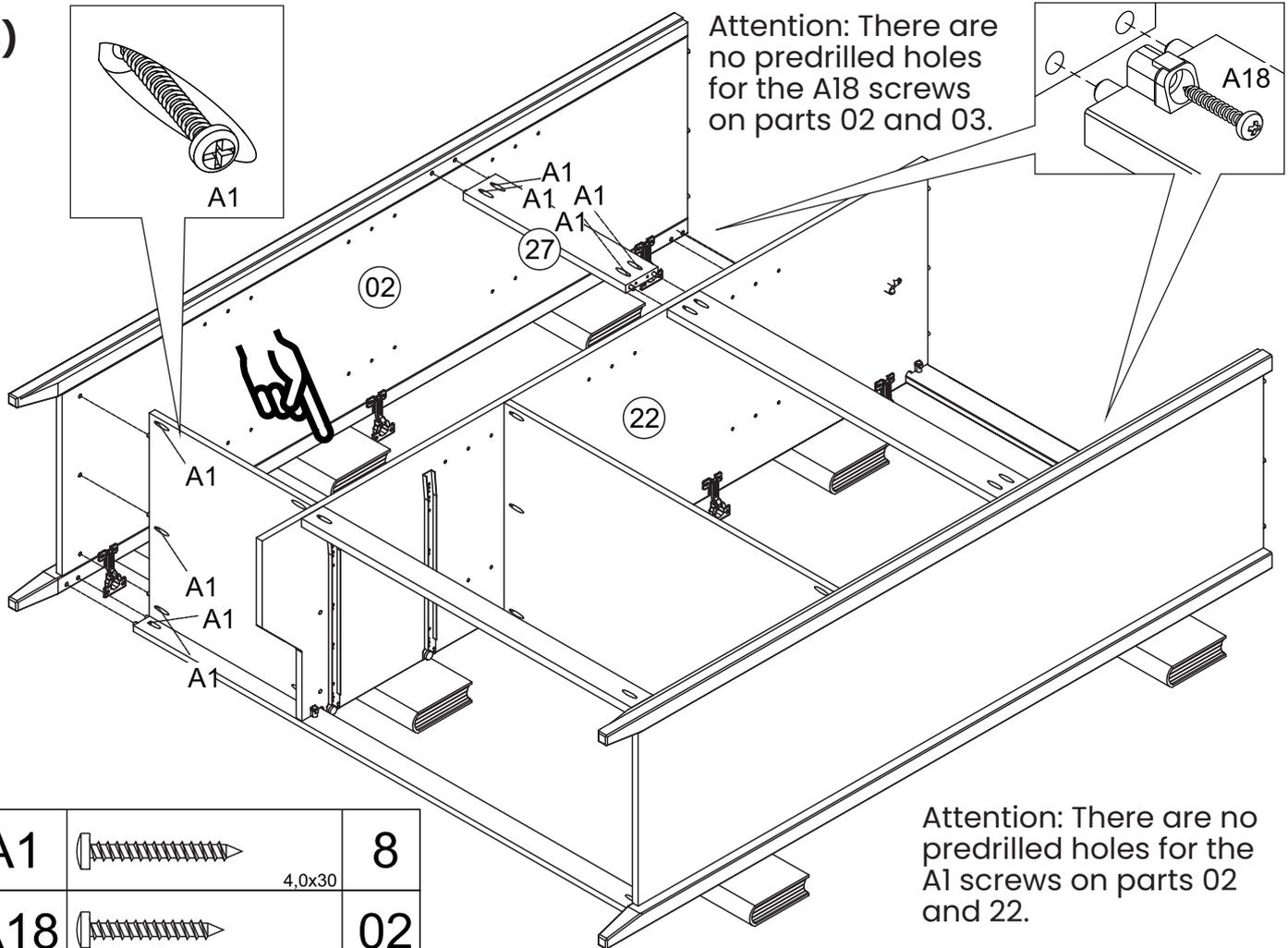
Attention: There are no predrilled holes for the A18 screws on parts 02 and 03.
