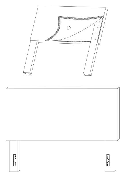
Stand the unit upright, adjust the legs on one level, then tighten all bolts.
