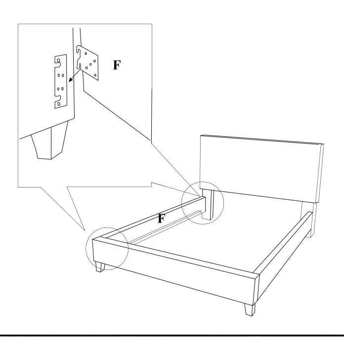
For making the entire unit assemble straightly, do not roll screws too tight when first secure the screw 80% is fine, after finish all screws, secure them completely and tightly.
