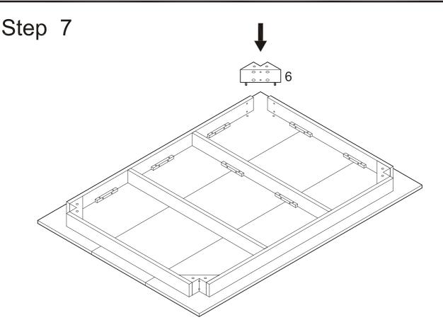
Attach corner blocks (6) to the table top using dowels as guides. Note that the glued surface of each corner block (6) will rest against the table top.
