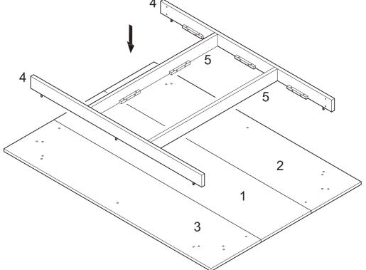
Attach the apron assembly from the previous step to the table top using dowels as guides.
