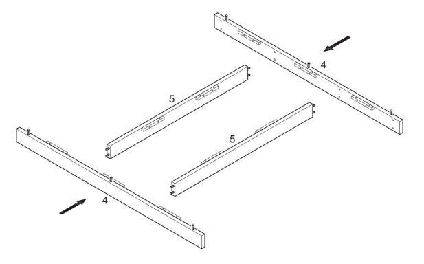
Attach inner aprons (5) to long aprons (4) using dowels as guides.
