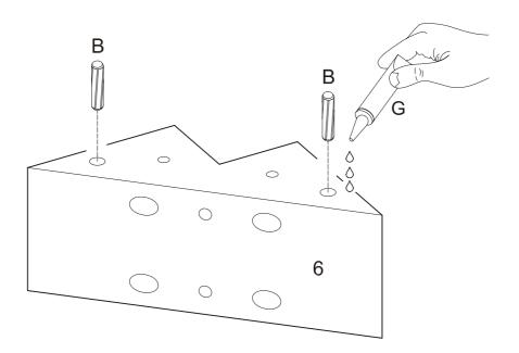
Insert dowels (B) into corner block (6). Apply glue (G) to the surface of corner block (6). Repeat this step for all corner blocks (6).
