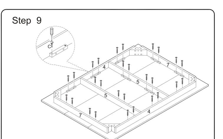
Secure aprons (4,5,7) to the table top using screws (C). Tighten screws (C) with a screwdriver.
