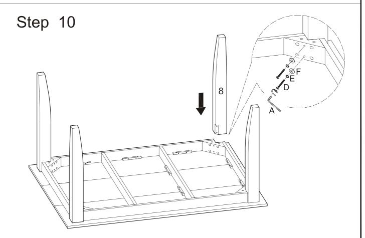
Attach table legs (8) to the table top assembly using bolts (D) and washers (E,F). Tighten bolts with wrench (A).
