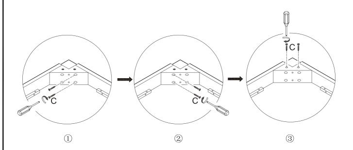
Secure corner blocks (6) to the table top assembly using screws (C). Apply pressure from the outside of the apron pieces while tightening screws (C) with a screwdriver.
