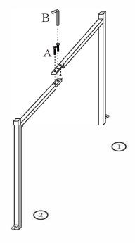
Join Half-Leg Sections (1 & 2) using Screw (A) as shown. (Note: for part (1) insert screws into first 2 holes closest to the horizontal end.)
