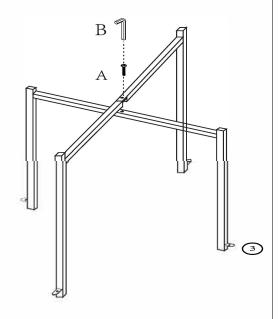
Place joined Leg Sections (1 & 2) from STEP 1 over Leg (3) as shown and align the screw holes. Next, use Allen Key (B) to drive Screw (A) to fasten the legs.
