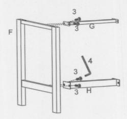
Assemble Stool Metal Cross Bar (G). Stool Bottom Metal Support Bar (H) to Stool Metal Side Frame (F) by using Short Bolt ③ as shown. Tighten by using Allen Key ④.
