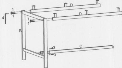
Assemble Metal Cross Bar (D). Bottom Metal Support Bar (C) to Metal Side Frame (B) by using Long Bolt ①, Short Bolt ③ as shown. Tighten by using Allen Key ④.
