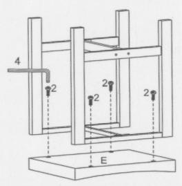
Install Stool Top Panel (E) to Assemble Unit by using Middle Bolt ② as shown. Tighten by using Allen Key ④.
