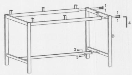
Assemble Metal Side Frame (B) to Assembly Unit by using Long Bolt ①, Short Bolt ③ as shown. Tighten by using Alley Key ④.
