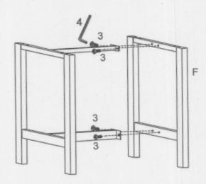
Assemble Stool Metal Side Frame (F) to Assembly Unit by using Short Bolt ③ as shown. Tighten by using Alley Key ④.
