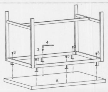
Install Top Panel (A) to Assemble Unit by using Short Bolt (3) as shown. Tighten by using Allen Key (4).
