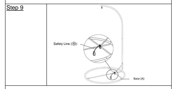
Insert the Carabiner on the Safety Line(10) into the Base(A), and screw up the Carabiner. Your Hanging Chair Base is ready for use.
