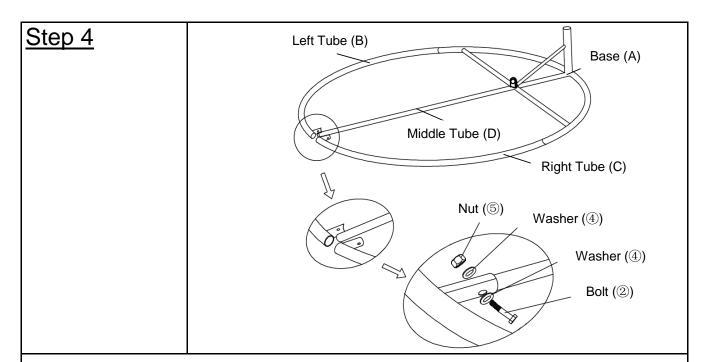
Attach Lett Tube(B) and Right Tube(C) to Middle Tube(D) using Bolt(2) and Washer(4) on one side, and using Washer(4) and Nut(5) on the other side; tighten with Spanners(12) and Spanner (13).
