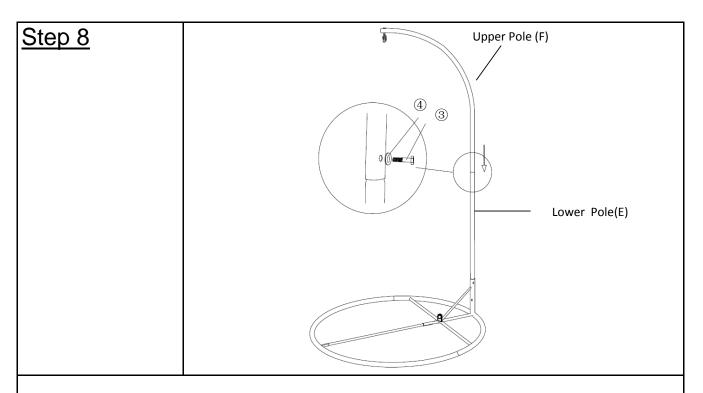
Insert the Upper Pole(F) into Lower Pole(E) and align mounting positions. Insert Lower Pole(E) into Base(A), turn the Lower Pole(E) and align mounting positions. Attention the Lower Pole(E) and Upper Pole(F)'s screw holes need to backward. Attach Upper Pole(F) to Lower Pole(E) using Bolt(3) and Washer(4) with Spanner(12) . Now, tighten all Bolts and Nuts at all joints sequential manner. Place Bolt Caps(6) on Bolts and Nut Caps(7) on Nuts(5).
