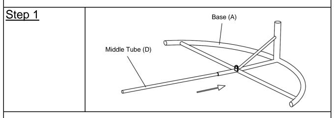
Place the Base(A) and Middle Tube(D) on a clean, non-marring surface. Insert Middle Tube(D) into the Base(A) as pictured.
