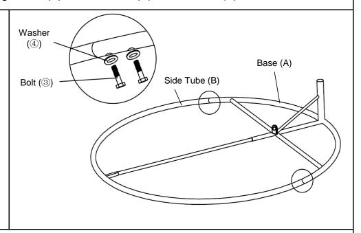
Attach Right Tube (B) and Left Tube (C) to Base (A) using Bolts (③) and Washers (④), with Spanner(12).
