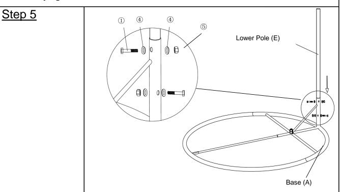
Insert Lower Pole(E) into Base(A), turn the Lower Pole(E) and align mounting positions. Attention the Lower Pole(E)'s screw holes need to backward.
