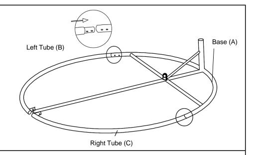
Place the Base(A), Left Tube(B) and Right Tube(C) on a clean, non-marring surface. One by one insert Right Tube(B) and Left Tube(C) into the Base(A).
