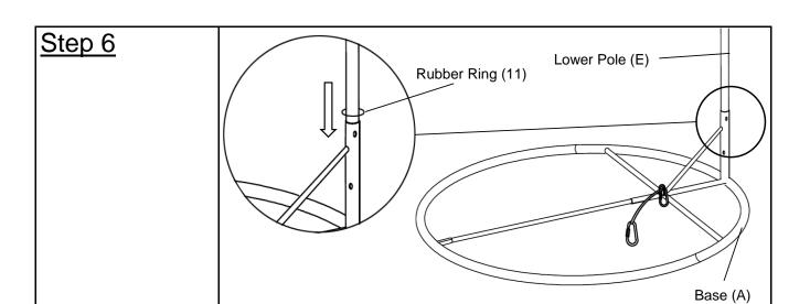
Move the Rubber Ring(11) down the Lower Pole(E) until it is flush with the top of the Base(A).
