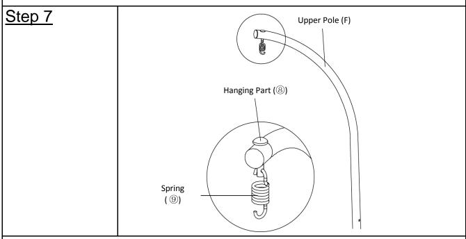
Insert Hanging Part(®) into the top of Upper Pole(F). Then insert the Spring(®) into the Hanging Part (®).
