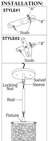
¶ o Refer to the mounting bracket style that matches the bracket that is included with your fixture. Attach the mounting bracket to the outlet box using electrical box screws (not included).
