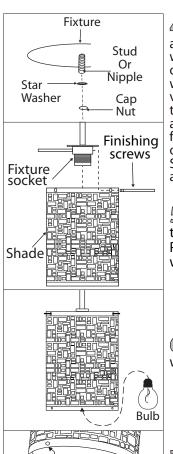
Once connections of wires are completed, carefully tuck wires and wire nuts into the outlet box making sure no bare wire (on the black and white) is visible at the wire nuts. Install the light fixture to the wall by aligning the hole(s) in the fixture with the studs or nipple on the mounting bracket. Secure in place with cap nut(s) and star washer (s).
