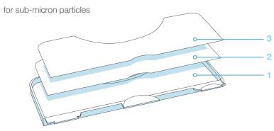
Use the cleaning tool to brush dust off the filters. It is recommended that you change Junior's filters every 6 months, depending on the frequency and intensity of his cleaning.
