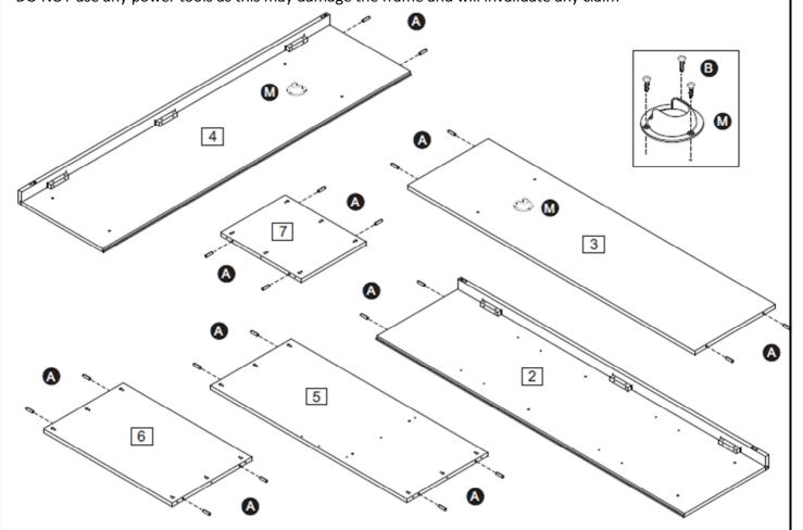
Step 4: Insert hardware part N to the right panel (2) and centre panel (3) using a small mallet (not provided). DO NOT use any power tools as this may damage the frame and will invalidate any claim
