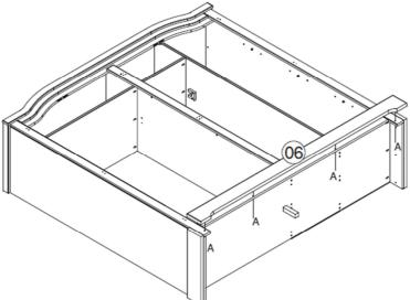
Step 12: Secure the top frame using hardware part P and a screwdriver (not provided). DO NOT use any power tools as this may damage the frame and will invalidate any claim.
