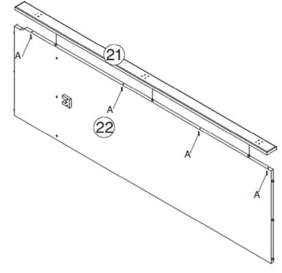
Step 5: Connect the left division panel (22) and right division panel (28) to the small top shelf (23) using hardware part A and a screwdriver (not provided).
