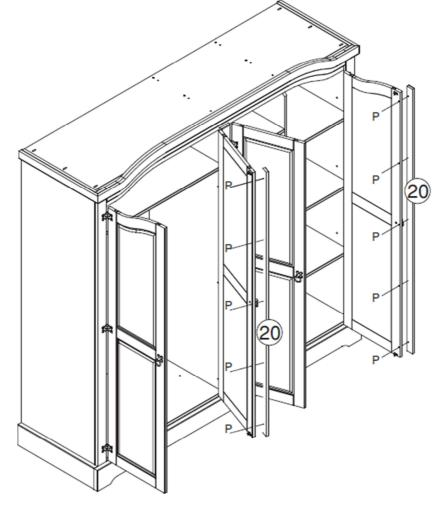
Step 20: Attach the back panels (9), spine (16) and right back panel (29) using hardware part E and a small mallet (not provided).
