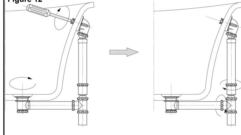
12 - Attach the Drain Plug and Water Overflow Cap to the bathtub. Make sure the opening on the Water Overflow Cap is facing downwards.
