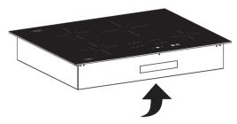
Serial plate is located at the front edge of the burner box of the cooktop.
